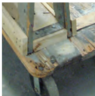
Wood—splinters and rot
