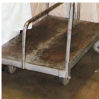
Metal—dents and rusts
